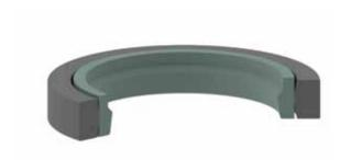
K704 is two piece single acting rod seal which consists of one special mixture PTFE profile ring and a NBR elastomer ring as energizing element.
