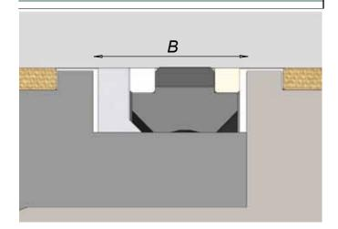
If a back up ring is used in unpressurized side, the seal could resist up to 1500 bar static pressure.
