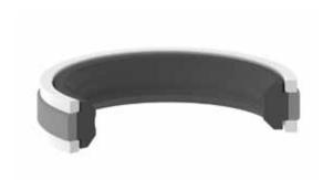
K48 is a four piece double acting heavy duty piston seal which consists of one TPE profile ring, one elastomeric nitrile rubber to pre load sealing element and two thermoplastic back-up
