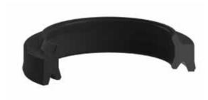
K106 is a single acting pneumatic wiper ensuring that foreign particles do not penetrate into the pneumatic cylinders. The lip is designed in a particular way that it functions as a rod seal and wiper.
