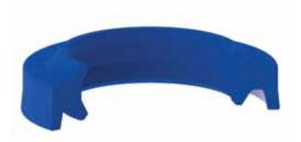
K103 is a single acting double wiper ensuring that foreign particles are not introduced into the hydraulic cylinders. The lip is designed in a particular way that it reliably wipes off the dirt but leaves a residual oil film on the rod.
