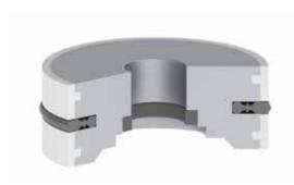
K61 is a double acting pneumatic compact seal which consists of two POM guide rings, one NBR sealing element (dynamic and static) and an aluminium body.
