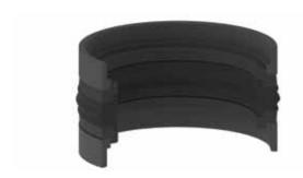
K518 is a five piece double acting compact seal which consists of one elastomeric nitrile rubber sealing element, two polyester elastomer back-up rings on both sides to prevent extrusion into the sealing gap and two special profiled guide rings produced from thermoplastic to absorb transverse forces.
