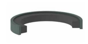
K762 is a two piece double acting piston seal which consists of one special mixture PTFE profile ring and a square ring as energizing element.
