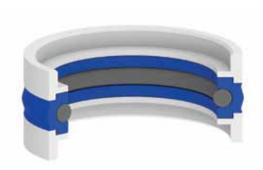
K46 is a four piece doble acting compact seal consisting of polyurethane sealing ring with NBR energizer O-ring and two special profile guide rings made of thermoplastic to absorb transverse forces.
