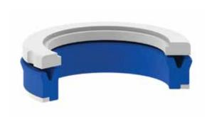
K44 is a three piece single acting sealing set which consist of one main sealing component, one thermoplastic back-up ring and one POM piston ring.
