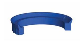
K101 is a single acting wiper ensuring that foreign particles are not introduced into the hydraulic cylinders. The lip is designed in a particular way that it reliably wipes off the dirt but leaves a residual oil film on the rod.
